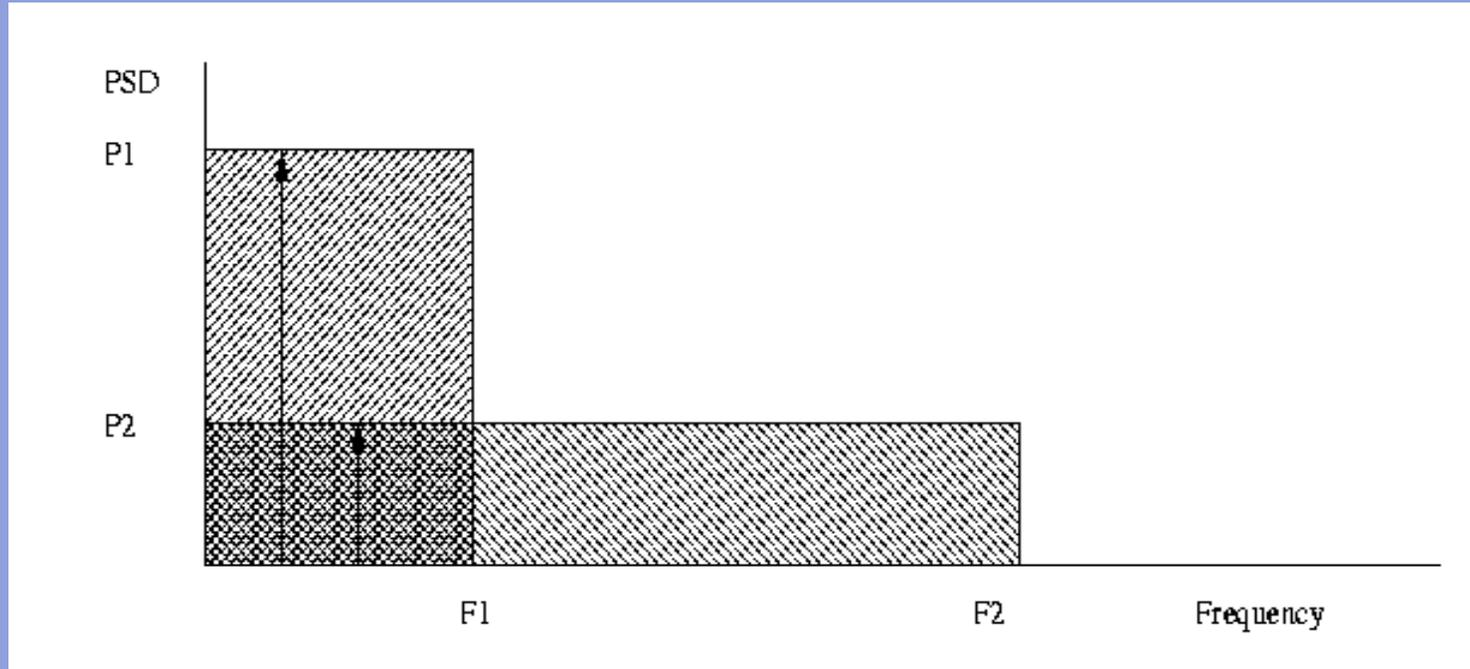
Very high sampling rate ADC with very poor resolution (1 bit)
