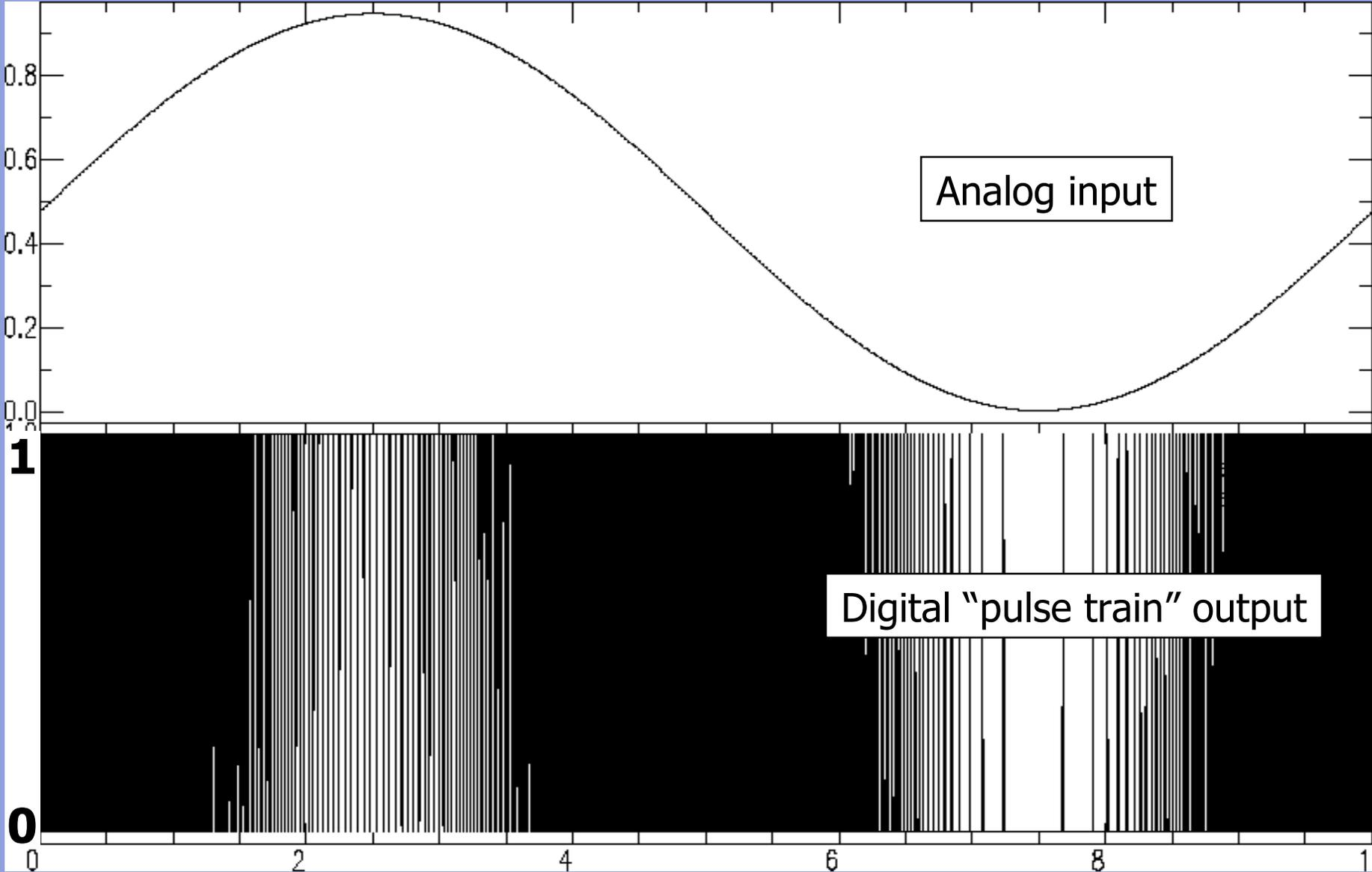
Very high sampling rate ADC with very poor resolution (1 bit)
