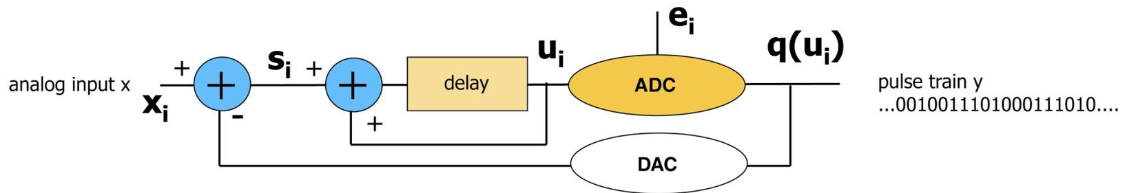
$$\left. \begin{aligned} s_i &= x_i - q(u_i) \\ u_i &= s_{i-1} + u_{i-1} \\ q(u_i) &= u_i + e_i \end{aligned} \right\} q(u_i) = x_{i-1} + \underbrace{(e_i - e_{i-1})}$$
