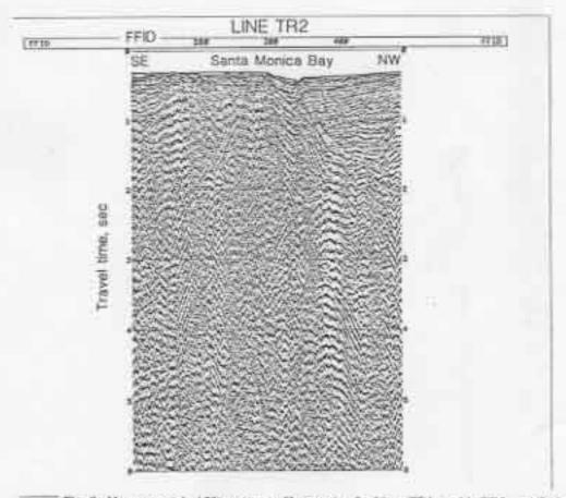
Fig. 9. Near-trace (ch. 150) constant offset section for Lines TR1a and b, TR2, and TR3. As described in text processing included band pass filtering, automatic gain control (AGC), and water column mate.
