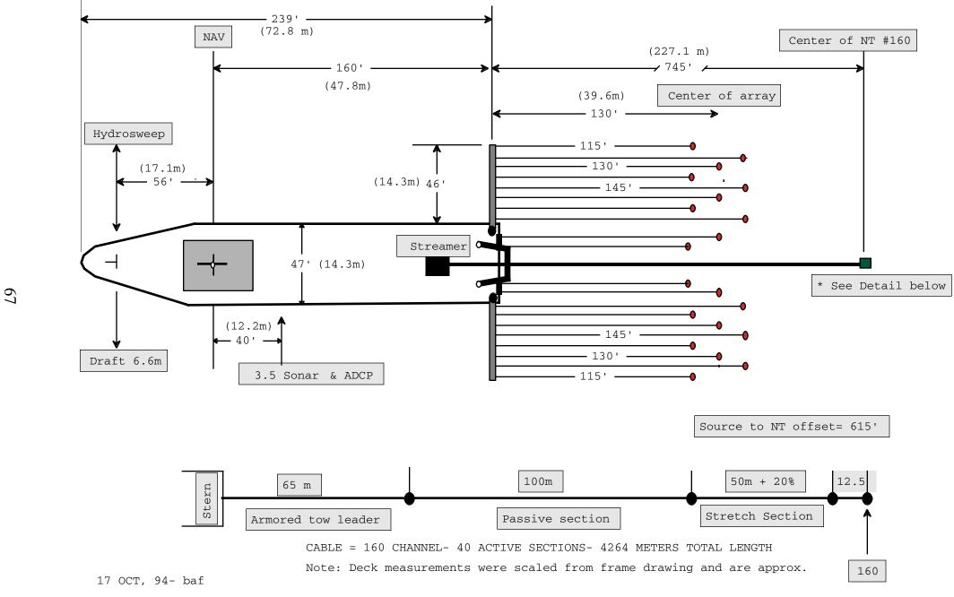
Fig. 3. Schematic diagram of **R/V Maurice Ewing** showing air gun and streamer deployment geometry.
