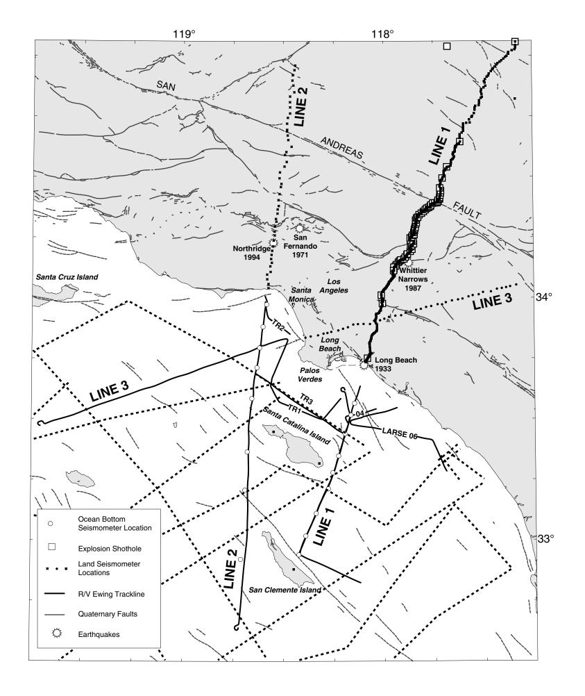
Fig. 1a. Map presenting an overview of offshore-onshore part of the LARSE experiment, showing locations of LARSE lines 1 to 6, and transit lines TR1 to TR3. Ocean Bottom Seismometer locations along lines 1 and 2 are shown as unfilled circles. Detailed view of land phase of LARSE along line 1 is also shown.
