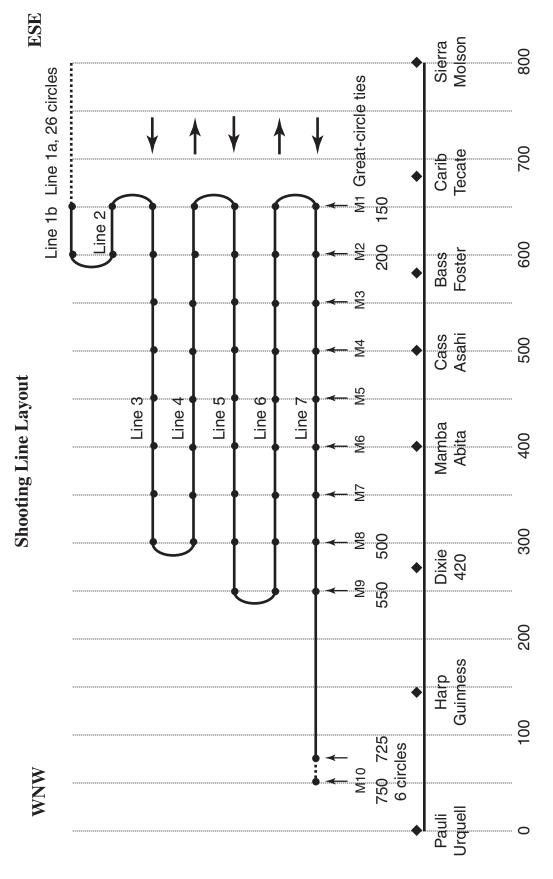
Schematic of shooting pattern along the main IPOD transect. Each new line number represents a switchback and change of direction. Shooting direction is indicated by arrows. Points labelled M were waypoints given to the bridge to maintain an approximate greatcicle path (the ship could only stear a rum line). Numbers along the bottom are distances from pauli in kilometers.
