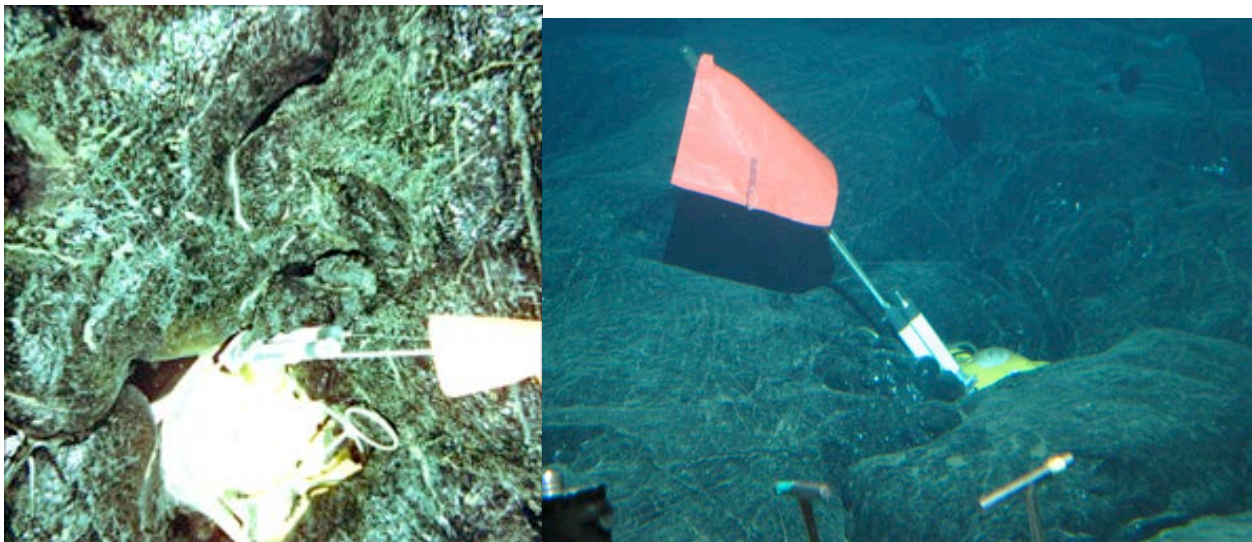
Near bottom photo of LC2000 buried in Lava using the WHOI TowCam aboard the R/V New Horizon (left – care of Dan Fornari). Photo of completely inundated LC2000 unit from lava flow (right – taken from Alvin). Note: both units shown were still in acoustic communication.
