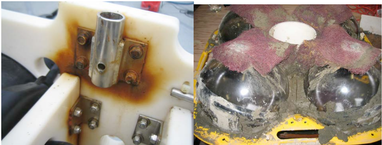
(Left) Enhanced corrosion of OBS hardware at OBS site 12. (Right) Excessive sedimentation observed in floatation hardhat at OBS site 03.
