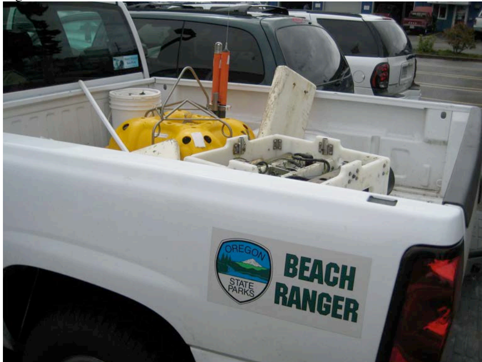
OBS unit recovered at Seven Devils State Park by Park Rangers. This unit was from OBS site 12 with a deployment depth of 103 meters and presumed to have been dislodged by a fishing net.
