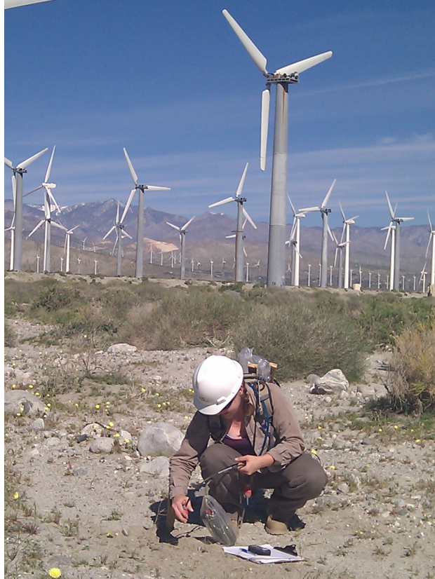
Student Kathy Davenport deploys a Texan seismograph on a wind farm near Palm Springs.
