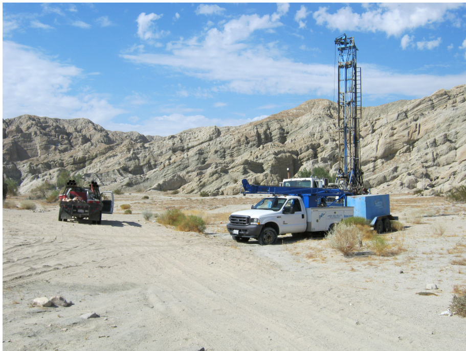
Rig and crew from Sam Crum Water Well Drilling Inc. drilling a seismic shot hole near the Salton Sea.
