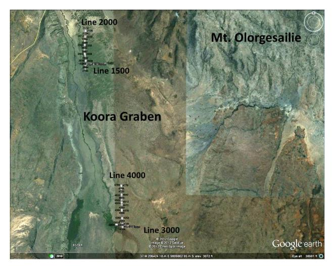
(magnetic profiling) in 2009 by Dr. John Githiri (University of Nairobi), which suggested thicker sedimentary deposits in those areas. In each of the two focus areas, two intersecting linear seismic reflection transects were acquired in roughly N-S and E-W orientations using a PEG-40kg Propelled Energy Generator seismic source. The source energy was recorded into 72
