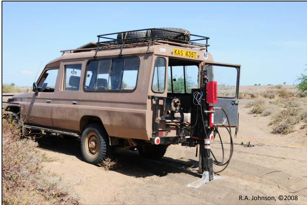
Figure 1. Hydraulic lift, nitrogen-gas-accelerated weight-drop seismic source mounted on the back of a Toyota Land Cruiser. Photo taken close to the end of Line 1, West Turkana seismic survey.
