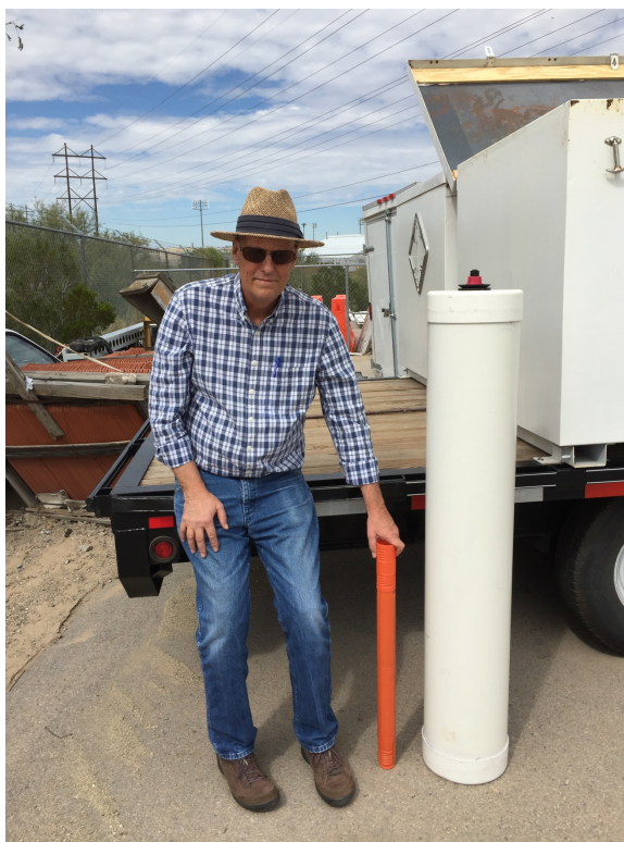
Figure 2. Industry size seismic cartridge on left. Crustal scale seismic cartridge on right. Crustal scale cartridge holds 200 lb. of emulsion at 1.25 g/cc.
