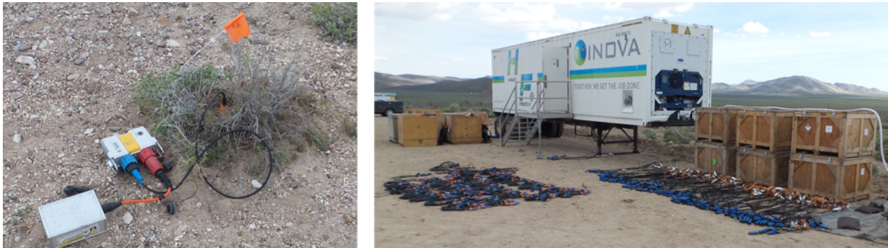
Figure 2. (left) Example of geophone deployment, battery, and digitizer. (right) Truck with field computer and racks for downloading data and charging batteries.
