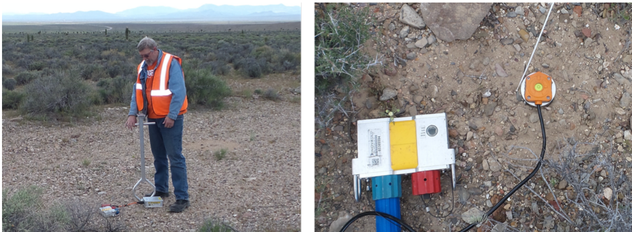
Figure 3(left) Jig used to orient horizontal geophones. A compass is in the handle. (right) Deployed Z component geophone and digitizer/disk storage unit. The sensor package consisted of geophones (either vertical or 3C), a battery, and digitizer/disk storage. Battery life was expected to be approximately two weeks. Disk storage was about two weeks for the 3C and one month for the Z component.
