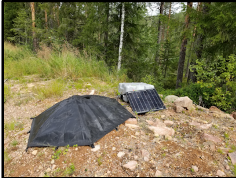
Figure 12. Example of an ARA installation with electronics enclosure, solar panel, and wind noise reduction dome visible. The acoustic sensor is below the dome. Note: due to photographic restrictions on the NNSS, this installation is from an unrelated project and is not an actual LSECE installation.
