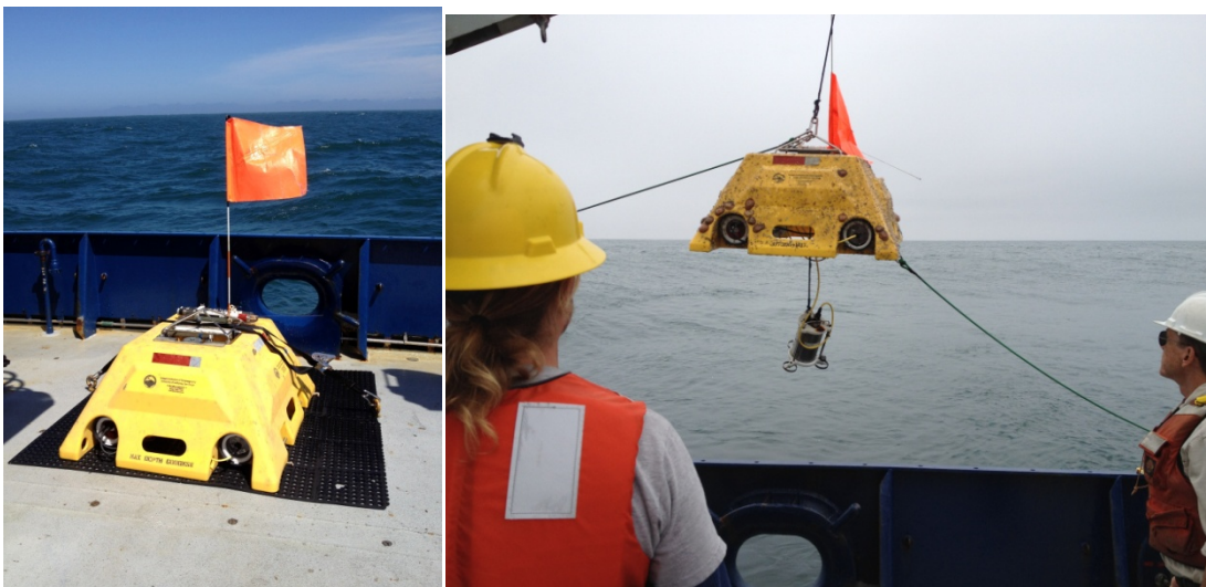
Fig 2: Pictures of SIO Abalone Ocean Bottom Seismometer once on deck and during the recovery procedures. Right shows seismometer instrument cylinder as tethered to the OBS frame.
