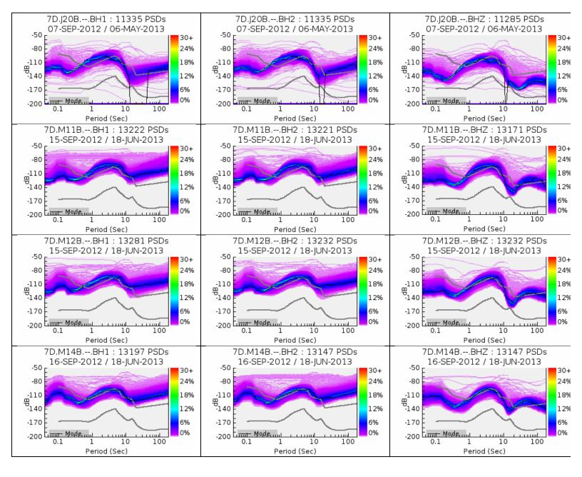
Appendix C (WHOI): Probability density function plots of power spectral density calculations for Year 2 WHOI stations. Each row represents two unoriented horizontal channels and one vertical channel for each seismometer. To eliminate noise from the initial settling of the instrument following emplacement, the plots only include data after the instrument has been deployed for two weeks.
