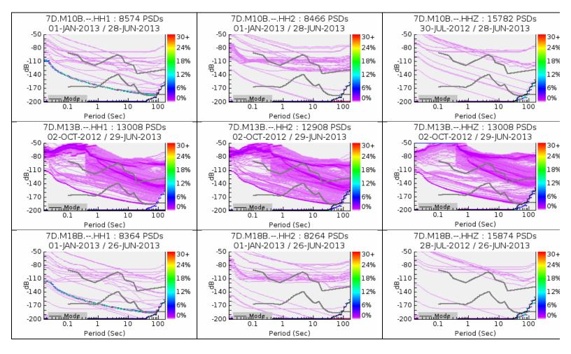
Appendix C (SIO): Probability density function plots of power spectral density calculations for Year 2 SIO stations. Each row represents two unoriented horizontal channels and one vertical channel for each seismometer. To eliminate noise from the initial settling of the instrument following emplacement, the plots only include data recorded after each instrument has been deployed for two weeks.
