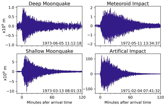
Figure 3. Examples of a deep moonquake, a meteoroid impact, a shallow moonquake, and an artificial impact. The events were recorded on seismic station S12 on the vertical component (MHZ). The timing for each event is in minutes and relative to the arrival time. The traces are displayed in displacement (in meters), with different scales for each event. The amplitude of the artificial impact signal exceeded the range of the instrument.
