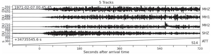
Figure 7. Data tracks provided in the miniSEED files. The top four traces show the components MHZ, MH1, MH2, and SHZ. The *x*-axis is the time in seconds after the P-arrival (1971-02-07 00:45:45) and the *y*-axis is in DU. The fifth trace, ATT, shows the timestamp. The *y*-axis is the number of seconds since 1970 January 1 (it is displayed with an offset of 34735545.6 s between 1970 January 1 and the arrival time).
