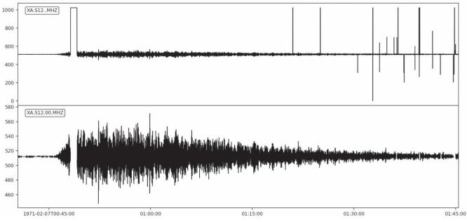
Figure 6. Data cleaning. The top panel shows the original data imported from the tape. The bottom panel shows the same data reimported, but excluding data with incorrect Barker codes (incorrect Barker codes indicate data frames that were not transmitted correctly). We have also removed single digital spikes from the trace (Figure 5 shows examples of these spikes).
