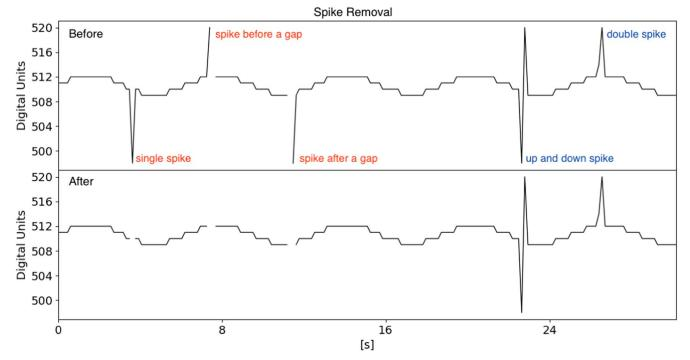
Figure 5. Digital spike removal. The top panel shows test data with added digital spikes, while the bottom panel shows the data after the spike removal process. The algorithm removes single spikes, spikes before a gap, and spikes after a gap. Up and down spikes and double spikes (which have two data points within the spikes) are not removed by the algorithm.
