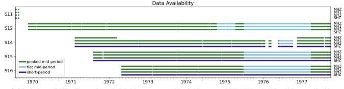
Figure 2. Seismic data availability. The experiments included three-component mid-period instruments (MHZ, MH1, and MH2), which operated in either peaked mode (green lines) or flat mode (light blue lines), and short-period instruments (SHZ; dark blue lines). We exclude S12's SHZ component (which was inoperative throughout the mission) and we partially exclude S14's MHZ component (which was inoperative for much of the mission).
