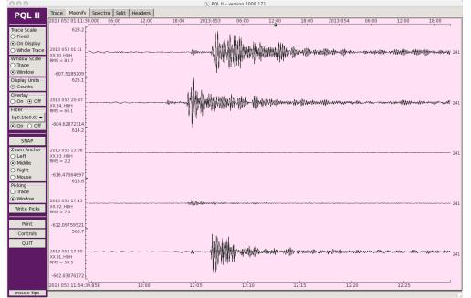
This plot shows the same data as in the figure above, but with each trace scaled to the maximum amplitude in that trace. The S wave is clearly visible on APG 2 and is arguably visible with S/N of  $\sim$ 1 on APG 3. The P wave is not observed on either 2 or 3.
