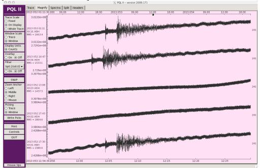
These are the same data as above but filtered to pass 0.02 go 0.1 Hz. Again, all traces are plotted with the same amplitude scale.
