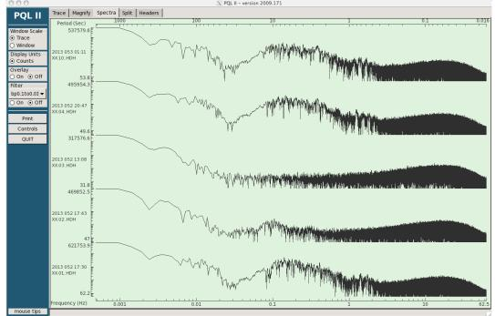
This figure shows the amplitude spectrum for each of the 5 APGs for a 24 hour time window that includes the earthquake shown above. The typical microseism peak and 50 s hump are seen on APGs 1, 4 and 10. They are not present on APG 3. On APG 2, the microseismic peak is not present and the 50 s hump is attenuated.
