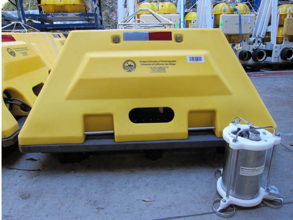
Figure 2. ABALONES unit attached to anchor (sitting on pallet in IGPP service yard). The Trillium-Compact sensor package is shown in front of ABALONES unit for perspective. In deployment mode, the sensor package is housed within the center well of the syntactic flotation-based frame and is mechanically detached from the main frame via corrodable link. At recovery, the steel anchor is left on the seafloor.
