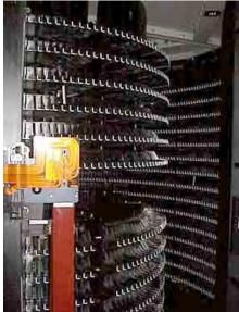
Figure 2. The Powderhorn Robot has room for 6000 tape cartridges with capacities up to 200 gigabytes each. As such the total capacity of this system can be more than 1 petabyte (1,000,000,000,000,000 bytes).
