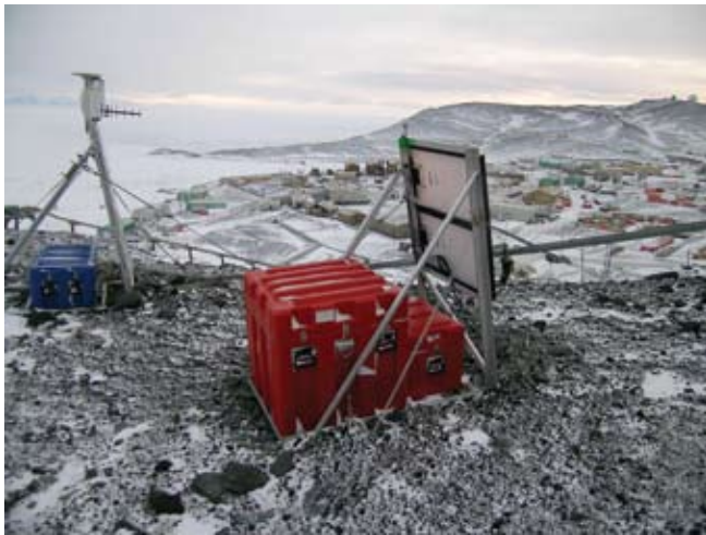
Figure A7.9. IRIS (center) and UNAVCO (left) cold station development testbeds overlooking McMurdo Station, Antarctica. These testbeds were used to proof MRI designs in field conditions in Antarctica (photo by T Parker).
