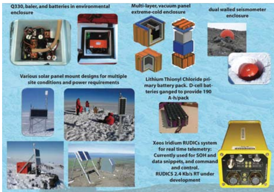
Figure A7.6. The work of the Polar Support Services engineers have allowed for vast improvements in low-power cold-rated, robust, super-insulated seismic systems for deployments in some of the harshest polar environments. All designs are available at http://www.passcal.nmt.edu/content/polar-design-drawing
