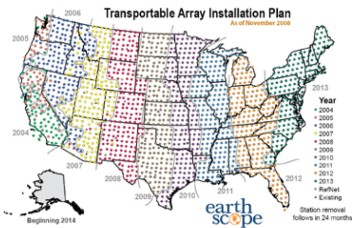
Figure 16. The map displays the current installation plan for the Transportable Array. Approximately 200 new stations are installed on the eastern edge of the array each year and approximately 200 stations on the western edge of the array are removed following a two-year period of operation.
