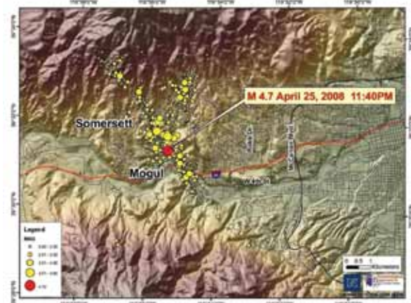
Figure 2. Double-difference relocated earthquakes of the Mogul, Nevada earthquake swarm. The mainshock had an M_w of 5.0, but a local magnitude M_L 4.7. The mainshock hypocenter was approximately 3 km depth. Hypocenters do not coincide with any known fault or geologic structure. Downtown Reno, Nevada is near the east edge of the image.
