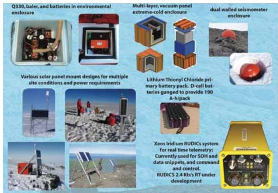
Figure A7.6. The work of the Polar Support Services engineers have allowed for vast improvements in low-power cold-rated, robust, super-insulated seismic systems for deployments in the some of the harshest polar environments. All designs are available at http://www.passcal.nmt.edu/content/polar-design-drawing
