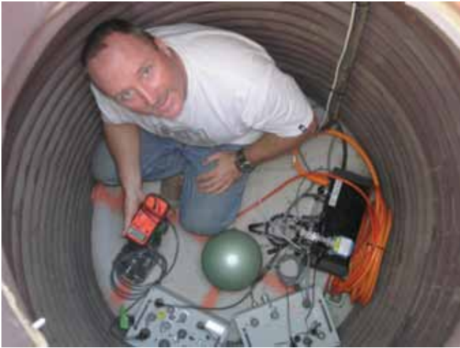
Figure A1.2. IDA field engineer installs the NGS equipment in a vault in Saudi Arabia (RAYN).
