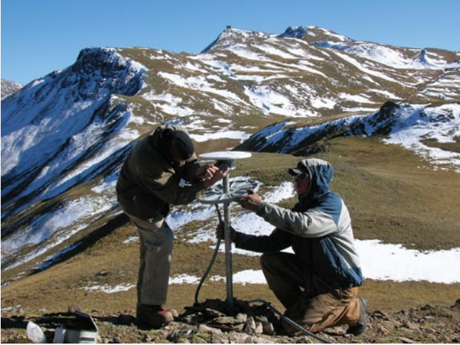
Figure 1.6. University of Colorado and UNAVCO personnel installing a campaign GPS stations near Silverton, Colorado. This station will be used to measure long-term deformation rates across the Rio Grande Rift.
