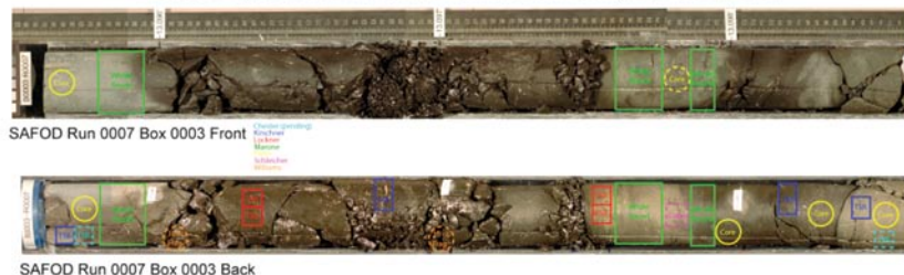
Figure 3.8. Photos of a section of core with samples selected by scientists for laboratory study (top) and the samples eventually distributed.
