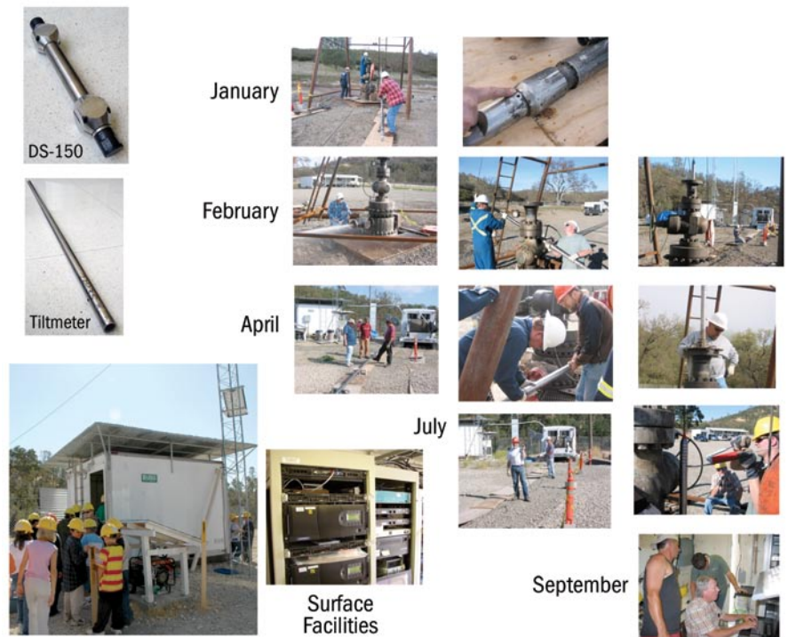
Figure 3.3. A collage of photos related to testing components of the downhole instrumentation systems and the surface facilities instrumentation facilities. A sixth grade class is shown touring the surface instrumentation building. The photo of the instrumentation rack shows the earthworm computers and LTO3 tape drives referred to in Volume I. The Geores recording system for the downhole seismometers is visible in the second rack.
