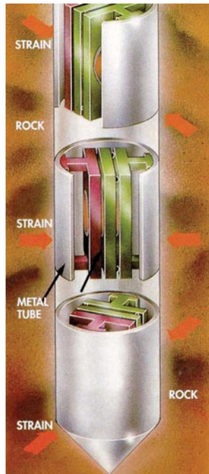
Figure 1.8. Schematic representation of a GTSM tensor strainmeter. The two green plates are a fixed distance apart. The red plate moves relative to the green plates as the borehole deforms.
