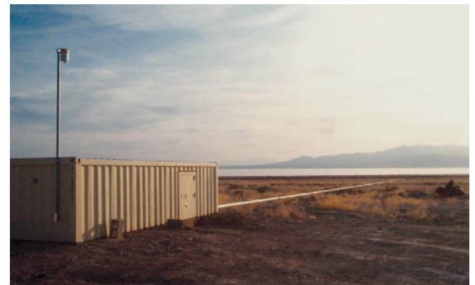
Figure 1.10. Long baseline laser strainmeter DH2 on the west side of the Salton Sea. The cargo container houses electronics and laser and a pad for the deep optical anchors. The long tube to the right is a vacuum tube through which the laser beam travels to a retro-reflector approximately 500-m away.
