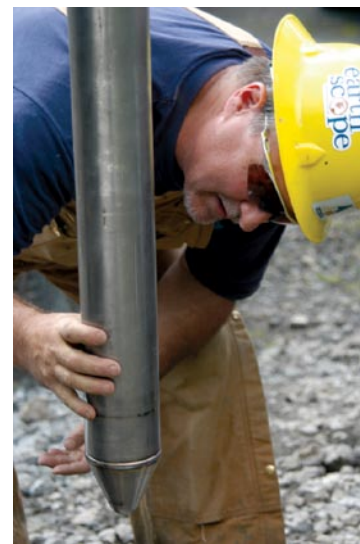
Figure 1.9. UNAVCO engineer installing a three-component seismometer in a PBO borehole.
