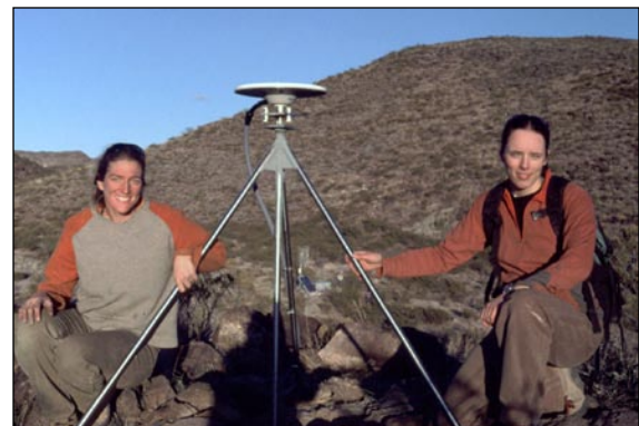
UNAVCO field engineers Beth Bartel and Nicole Feldl after the completion of short-brace continuous installation of PDBG GPS within the Socorro Magma Body.
