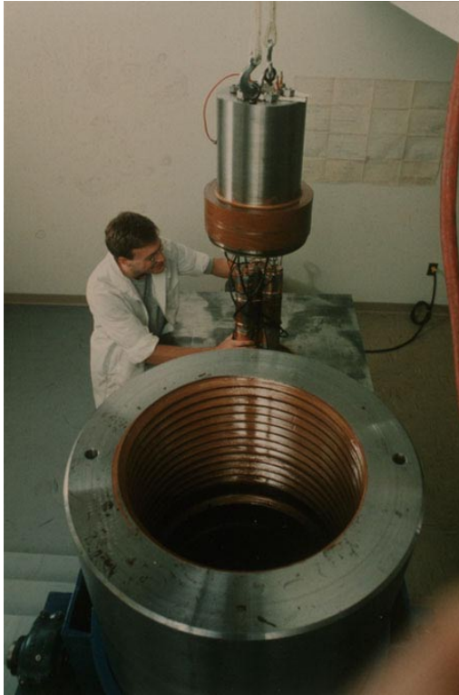
Pressure vessel capable of measuring velocities as functions of confining pressure, pore pressure, temperature and frequency.
