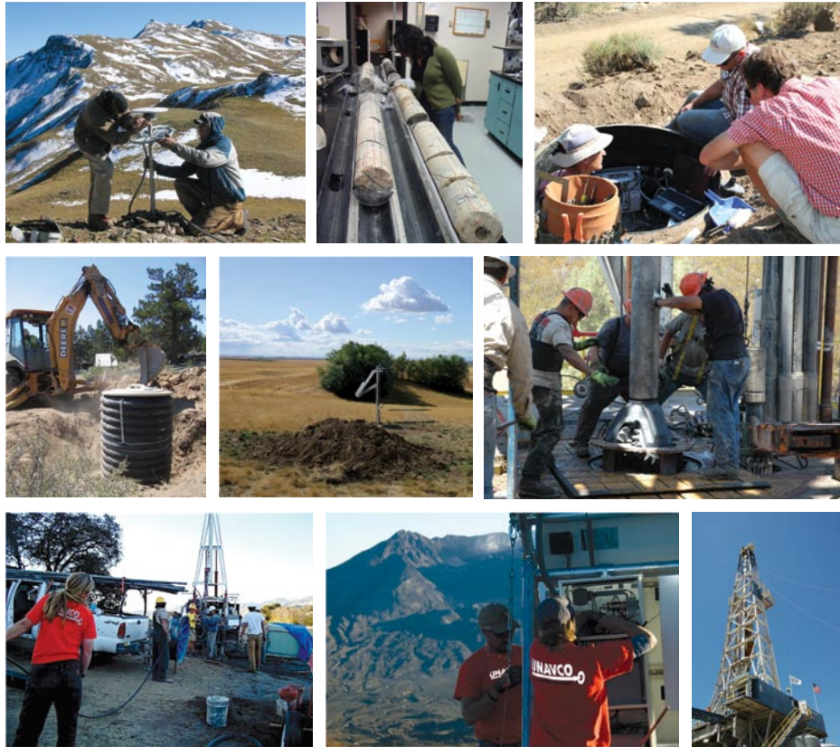
Figure 2.2. Top Row. (Left) Installing antenna for GPS station RG20 in the Rio Grande Rift. (Center) Core retrieved from SAFOD drill hole. (Right) Installing seismometer and supporting electronics for a typical Transportable Array station. Middle Row. (Left) Vault and site construction for Transportable Array station I05A near Bend, OR. (Center) Transportable Array station C08A near Almira, WA. (Right) Drilling of SAFOD observatory. Bottom Row. (Left) Installing PBO strainmeters near Parkfield, CA. (Center) Installing electronics for a typical GPS station. (Right) SAFOD drill rig.
