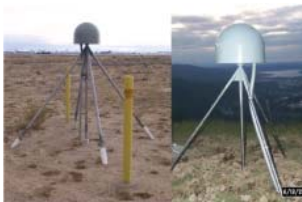
Figure II-2.11. A deep drilled (40-45 ft) monument at station SCIA in the SCIGN network (left) and a short drilled braced (6-10 ft) monument installed at station PUPU for the post-Nisqually earthquake response (right).
