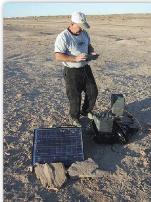
Figure 24. Aftershock deployment after Landers earthquake in Southern California.
