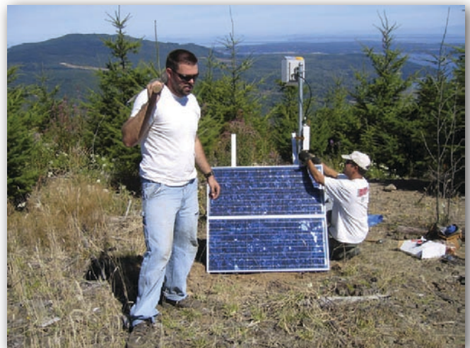
Figure 21. Radio telemetered broadband station on the Olympic Peninsula, above the Cascadia subduction zone.
