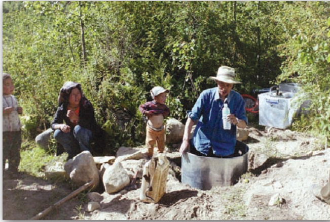
Figure 20. Installation of a broadband sensor vault in southeastern Tibet with local assistance.
