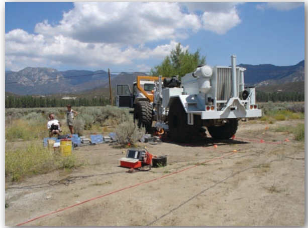
Figure 34. NEES vibrator deployed with PASSCAL multichannel systems in Garner Valley, California (Photo c/o Jamie Steidl, UCSB)
