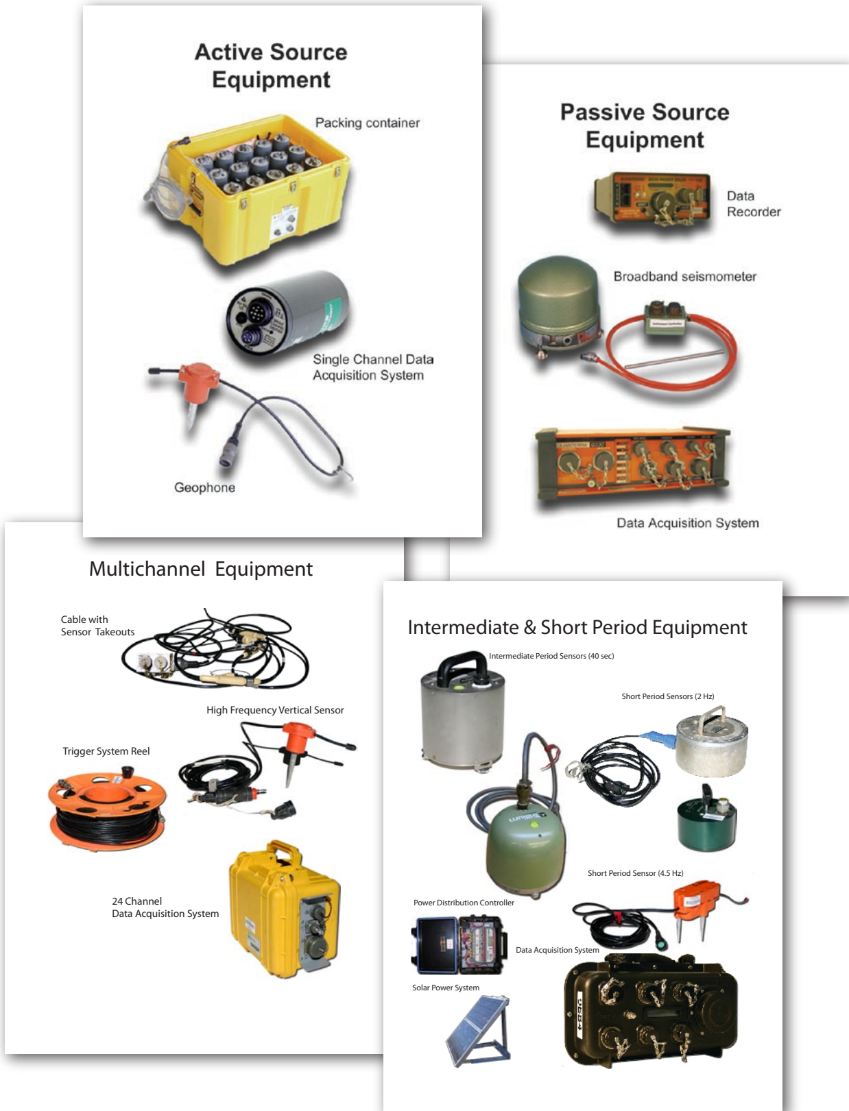
Figure 19. PASSCAL major equipment. Instrumentation provided and supported by the PASSCAL facility can be divided into four categories: active source, passive source broadband, intermediate and short period, and multichannel.
