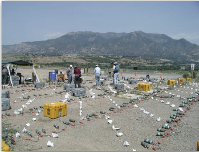
Figure 22. Single-channel TEXANs deployed in a dense array at Hill Air Force Base to image a toxic waste site.
