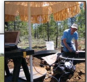
Jim Fowler installs an early TA station in California.
