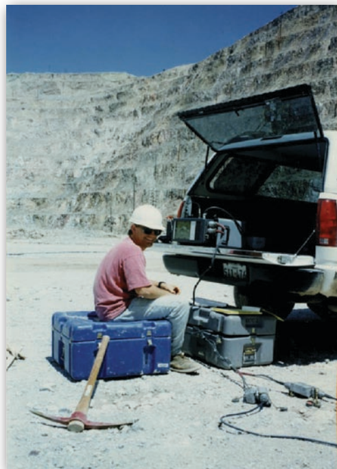
Figure 23. Multichannel system recording mining blasts at the Tyrone Mine, New Mexico.
