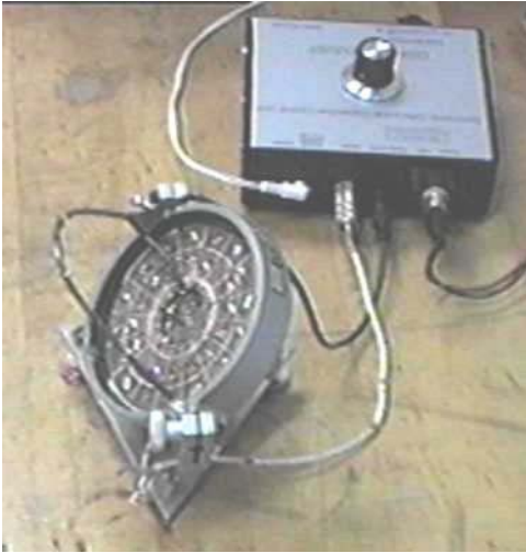
Figure 1. Photograph of the tilt-sensitive torsion pendulum, showing electronics support.
