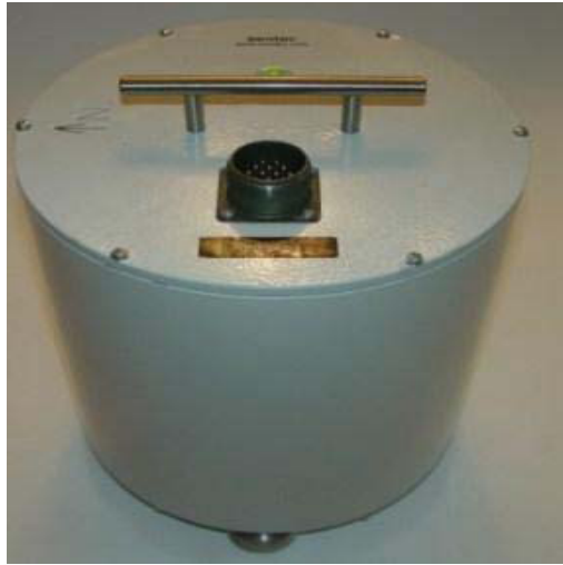
Figure 4: EEETEC EP-105 SEISMOMETER installed at all NNNSS stations
