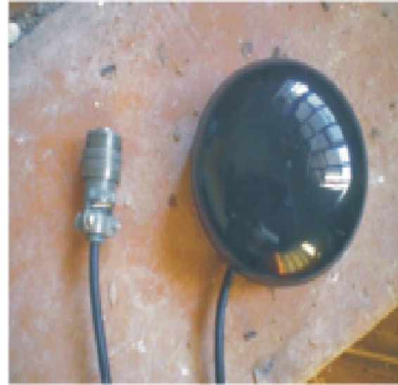
Figure 3: Time signal receiver for Timing system installed at NNNSS stations to get accurate time and for time stamping of the acquired seismic data.
